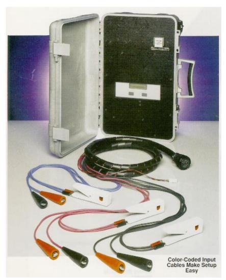
The new OM-170PL Series power logger is a rugged, dedicated datalogger pre-programmed for measuring ac parameters and packaged in a weatherproof case. Two basic models are available: one for use with current probes with a 1 Amp output and one for use with current probes and a 5 Amp output. Both units have three voltage input channels capable of measuring 0 to 600 Vac and three current input channels for use with current probes.
